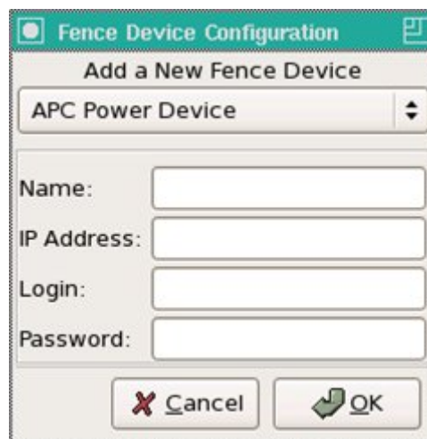
Figure 5: Setting Up Data Sharing Cluster - Defining Fencing Devices
